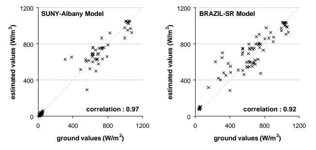
**Figure 1.** Scatter plot between hourly global solar irradiation estimates versus ground values measured in Caicó for January/2003. Only SUNY-Albany and BRAZIL-SR models are presented. Both models use the tri-hourly GOES-8 images to estimate solar irradiation.
