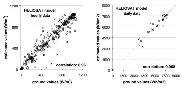
**Figure 3.** Scatter plot between hourly global solar irradiation estimates provided by HELIOSAT versus ground values measured in Caicó for January/2003. Either hourly and daily data were obtained using 12 METEOSAT images.
